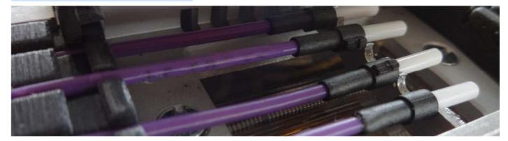
Cables and termini are easily loaded and securely held in the oven during the setup and cure process to ensure the best quality bond.
