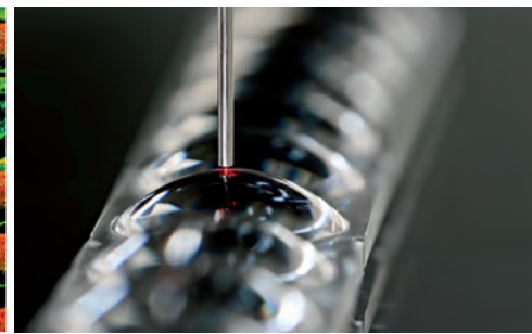
Micro-scale: Probe head with a diameter of only 50 µm (image left). Measurements in a 200 µm hole in a multi-layer circuit board and high-resolution 3D scan of the PCB surface (center images). Surface scans of a lens array (image right).
