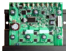
Compressor drive board included with the LCM series
