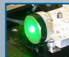
1 MHz piezo, 1 inch Φ 1 μs pulse excitation
