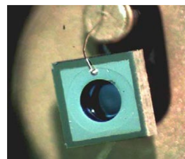
Figure 7. RAPD mounted on TO-18 header (SUR500S8)
