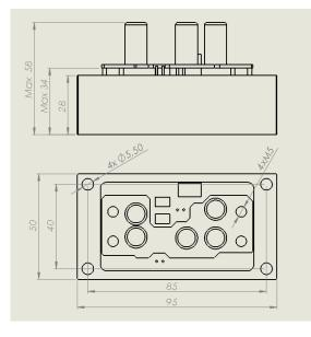
Dimensions of the Heatsink with 25V Capacitor Bank
