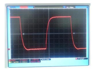
Current flowing through high power silicone diode. 62A 20kHz signal. Measured on sense resistor using current monitor output.
