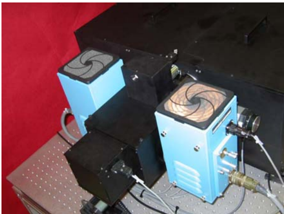
Two light sources (QTH and IR-emitter), reflective condenser, light chopper and filter wheel section
