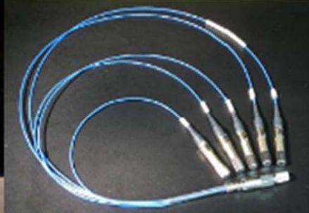
LRO Fiber Optics LOLA Flight Assembly
