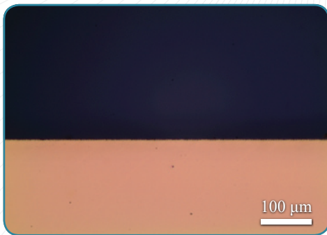
Figure 12. Non-tempered Eagle glass, thickness 0.4 mm. Top view.
