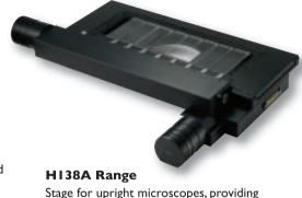
Stage for upright microscopes, providing an extended X axis travel range suitable for eight slides at 240x76mm. Stages can be configured with 2mm ball screws and 200 step motors for high speed applications and can be fitted with high precision encoders. H138A stages are pre-programmed with Intelligent Scanning Technology (IST) for improved metric accuracy.
