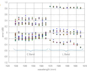
This figure illustrates the typical output power accuracy of standard ITLA lasers. The output power of each is recorded using a NIST traceable optical power meter. Measurements from each laser are taken at 10 different wavelengths for 7 different power settings. The data is taken from a random sample of 12 lasers.
