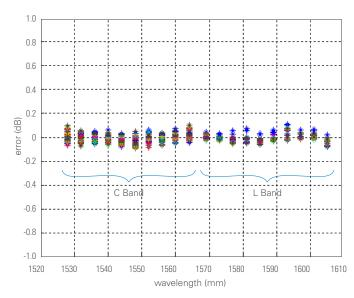
This figure illustrates the results of the same measurements, when the lasers are integrated into the IQTLS and controlled via the TIM application. The output power is now within 0.2dB across the entire range.
