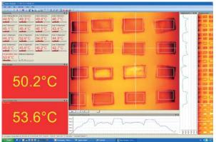
Example of linescanner function display layout
