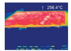
Processes can be examined thermally and deviating hot or cold positions are pinpointed automatically. Temperature distribution of a surface can be captured precisely within millisecond intervals
