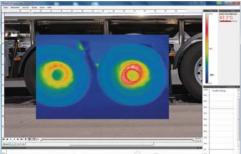
Lens of the thermal imaging camera determines the over all area of measurement displayed as a rectangular field of view
