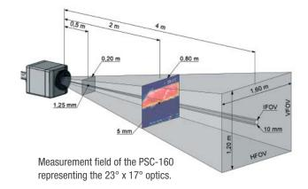
The measurement area (FOV) is determined by the appropriate lens selection, meanwhile the individual spot sizes are determined by the camera's detector resolution, e.g., 160x120 or 382x288.
