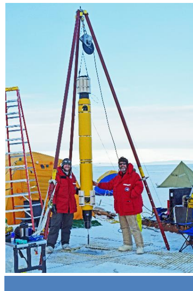
GA Tech used a 3.5 mm Linden STFOC tether on a NASA funded project to deploy a 10 ft long ROV under the Ross Ice Shelf in Antarctica capturing never before seen footage.
