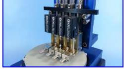
Multiple DART™ assemblies can be used in KrellTech and other manufacturers' connector polishers, converting these machines into mass bare fiber processing systems.
