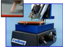
DART™ ferrule tips are designed so bare fibers can be polished at variable angles. The advancement feature maintains fiber contact with the polishing surface during entire process.
