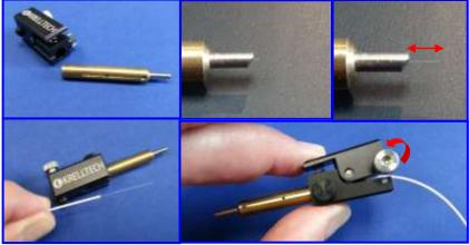
The patent-pending positioning feature, integrated in the common coupling mechanism, permits continual fiber advancement and retraction from the ferrule endface. This feature aids with fiber protrusion during polishing, attenuating transmitted power during system testing, and detector/transmitter proximity coupling control.
