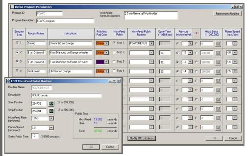
Scepter features an intuitive user interface for creating polishing programs. All polishing parameters including cycle time, pressure and speed settings are easily inputted for all connector types and desired surface geometries.
