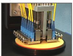
Scepter workholders feature Independent Suspension (IS) at each connector position for controlled pressure and uniform contact with the polishing surface. IS permits air polishing while maximizing film life. Each position is optically aligned for optimal polish geometry (patent pending).
