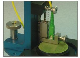
Proton<sup>™</sup> workholders feature Independent Suspension (IS) for controlled pressure and uniform contact with the polishing surface. The workholder is also optically aligned. for optimal polish
